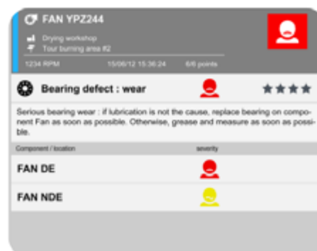
Detailed information on a defect with identified location
